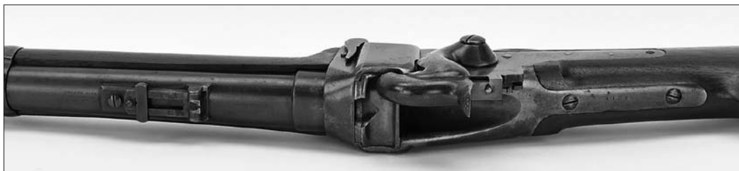
Zaklep sistema Sharps M 1859 (© Collectors Firearms).
